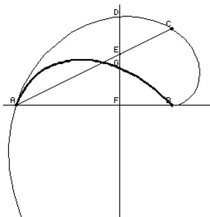
Figure 3. The graphs of  $[t \cos t, t \sin t]$ , a cord and another parametric curve
